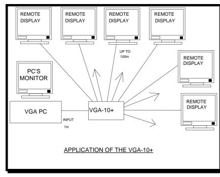
All connectors are on rear of case. Includes " Control" input and expansion output for tutor control of Autoswitch based classroom system. Turning the ControlSwitch (available from Calibre) On/Off enables/disables monitors connected via Calibre's AutoSwitch. Multiple VGA-10+s can be interlinked for large installations.
